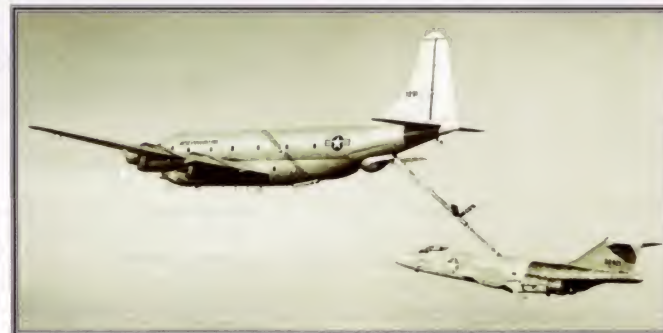
▲ More fuel The original Voodoos used the standard USAF refuelling boom, but were unusual in having a probe for a drogue system as well.
